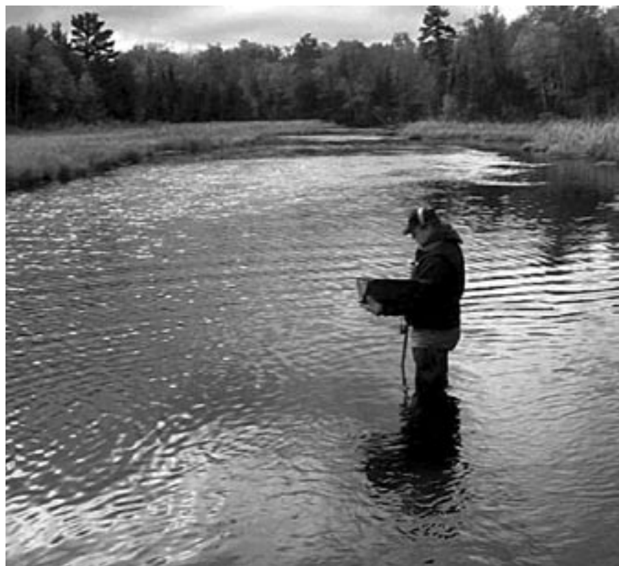
John Brown, Lac du Flambeau water resource technician, measures discharge to calibrate the stream gauge at Trout River. Photo courtesy of Lac du Flambeau Band of Lake Superior Chippewa.
